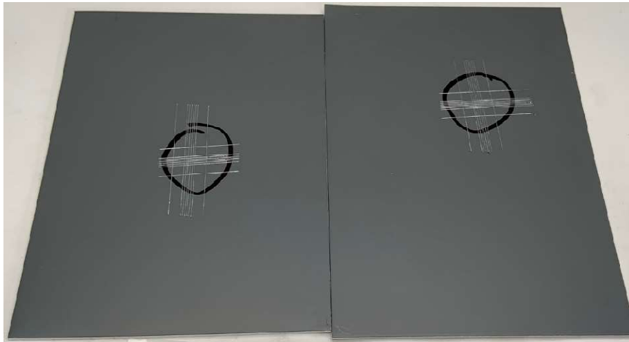
Figure 13 - Window Cleaner Resistance Panels 22 & 23
